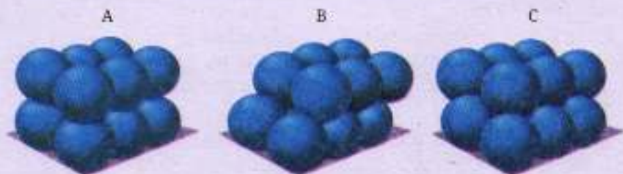
Fig. 14.17: These are some of the ordered ways of packing spheres in a cuboidal structure
